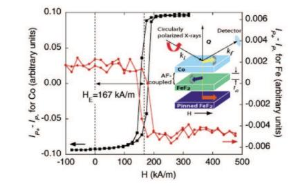
**Figure 2.** Hysteresis loops at Q = 0.49 and 0.38 nm<sup>-1</sup> for Co ( $\blacksquare$ ) and Fe ( $\bullet$ ) respectively. Inset: Representations of the X-ray experiment and sample.
