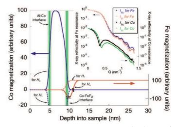
Figure 3. Spin density depth profiles for Co (blue) and Fe (red) spins obtained from the specular X-ray reflectivities (inset) at  $H_{\pm}=\pm796~\mathrm{kA/m}$ .
